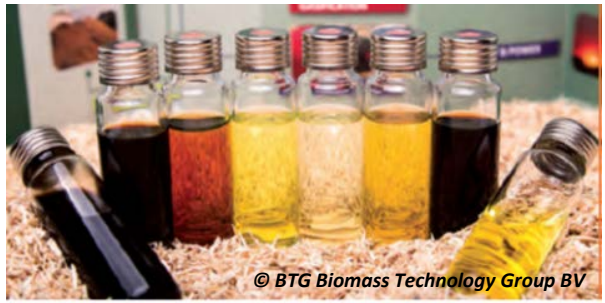
The full spectrum of biomass derived liquids from pyrolysis liquids (sides) to gasoline/diesel biofuels in the middle.
