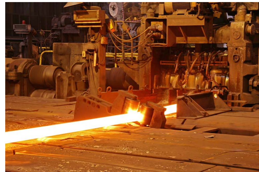
A heated billet passing through a rolling stand.
