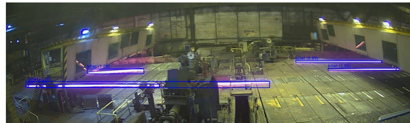
An object detection network trained solely with simulated data detects billets with high precision
