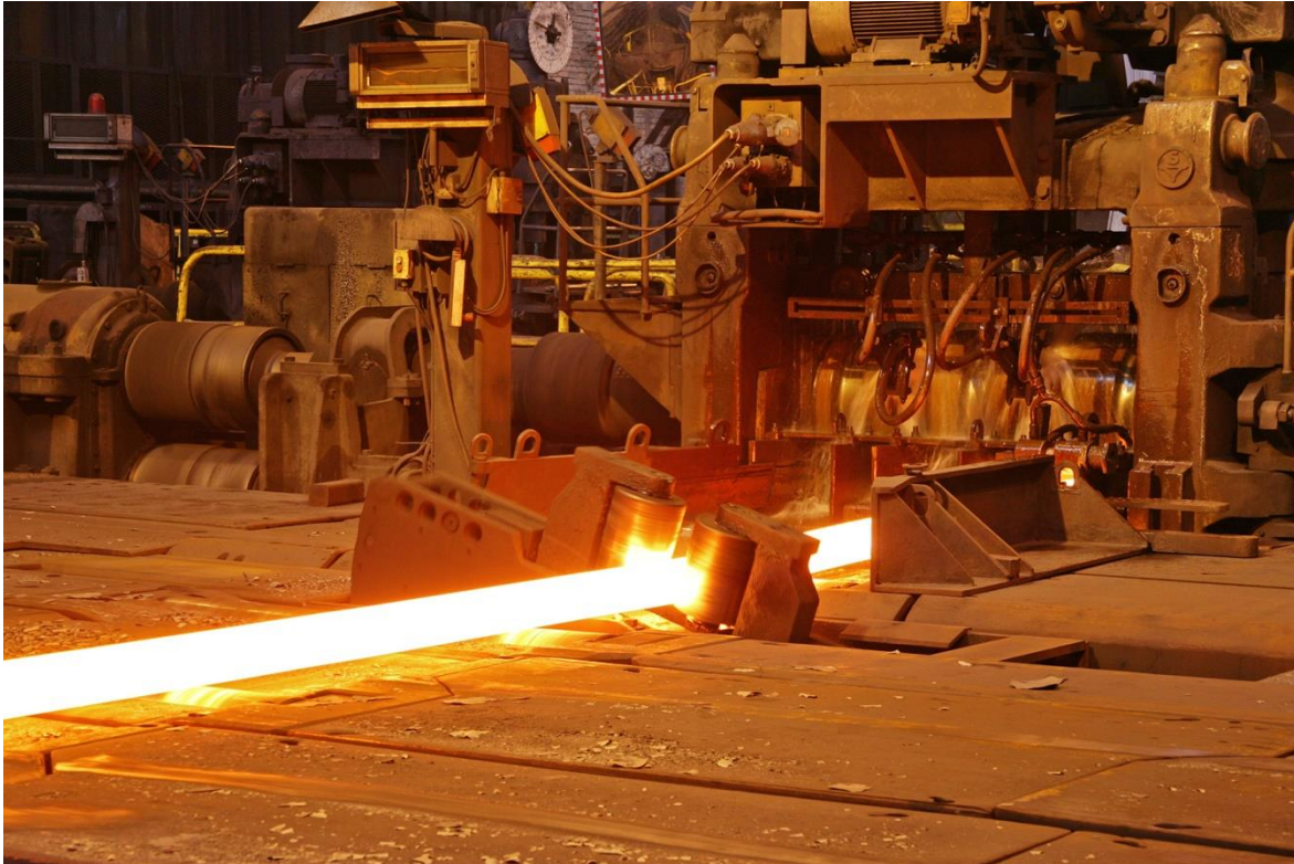
Figure 2: A billet passing through a rolling stand in the Nauweiler rolling mill
