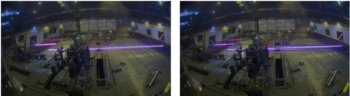
Figure 21: Left image: billet instance temporal segmentation without mask post-processing. Note that pixels of the same billet get wrong ID after the long gap. Right image: Billet instance segmentation with Mask-RCNN post-processing.
