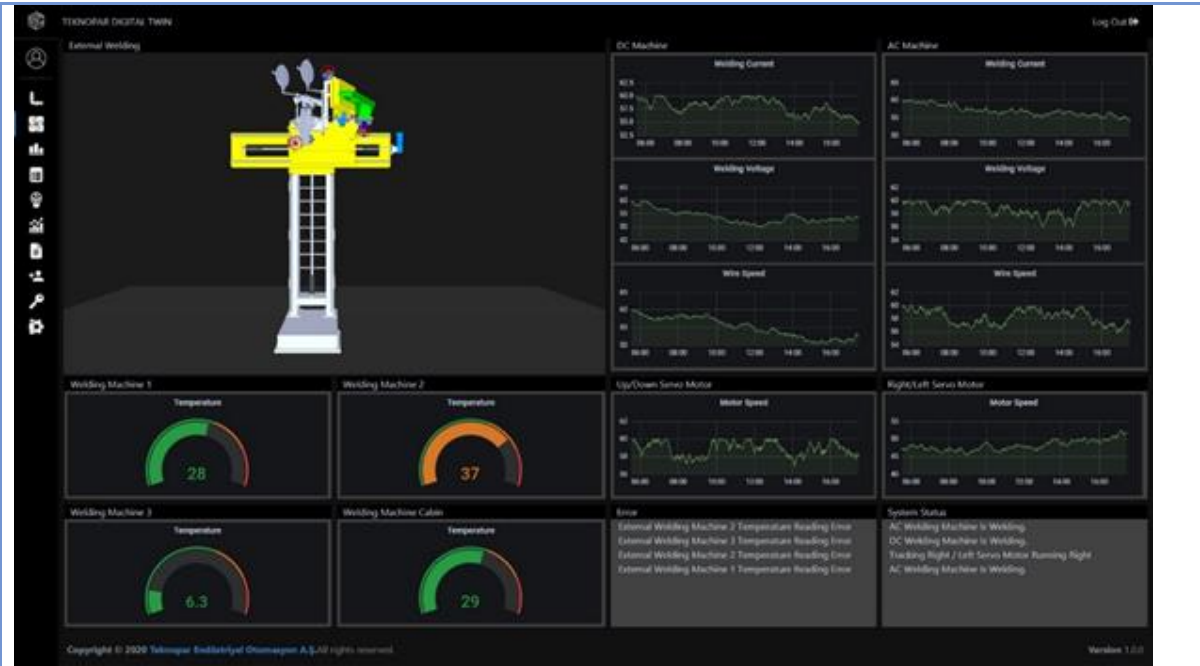
Figure 28: TIA UX Sample GUI for External Welding of SWP displaying Real-Time sensor Data.
