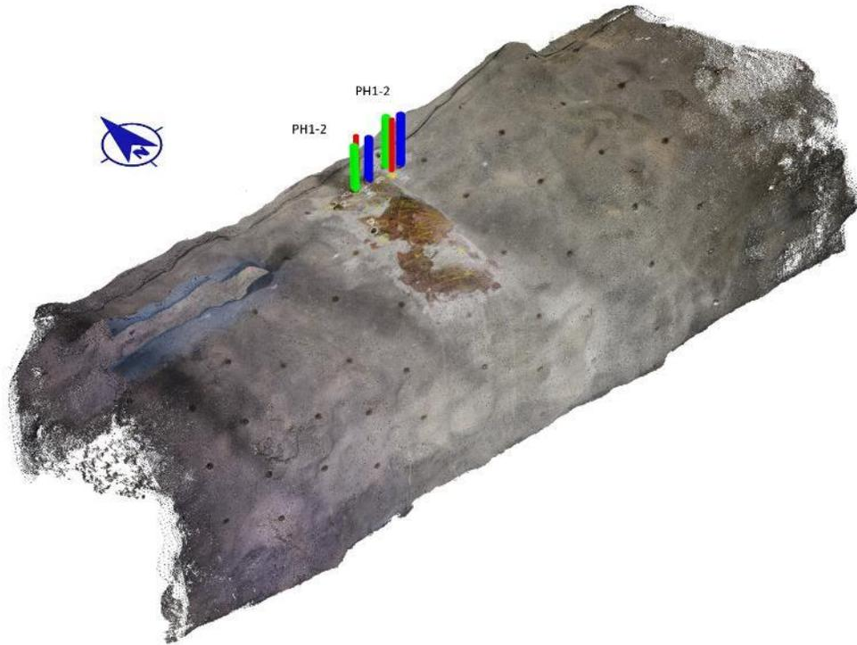
**ML2:** four *doble sidecoring* measurements, at two depths
