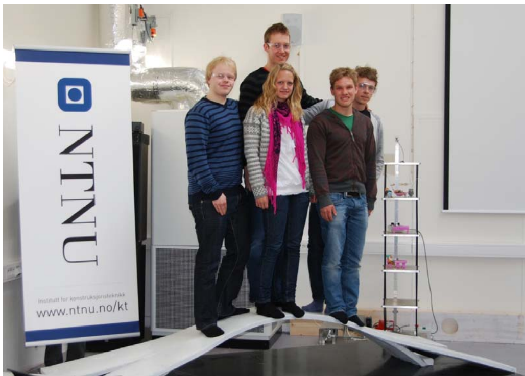
Da Vinci bridge made of super high-strength concrete, reinforced with steel fibres. The concrete was measured to have a compressive strength of 113.7 MPa.
