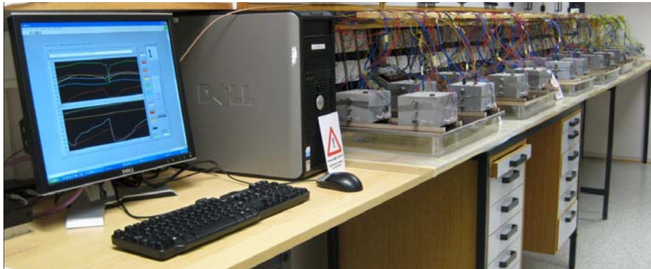
Dataloggers and concrete specimens used for the experimental work on chloride induced corrosion. Photo: Ueli Angst
