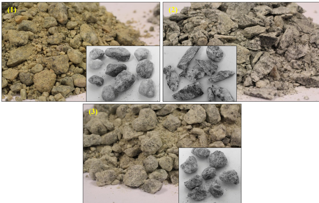
Different sand types: (1) High quality 0/8 mm natural sand from Årdal; (2) Low quality 0/8 mm by-product of coarse crushed aggregate production (should not be called manufactured sand); (3) High quality 0/8 mm manufactured sand
