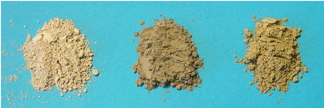
Ground limestone, fly ash and clinker – components in cement
