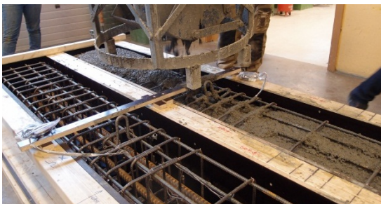
Reinforcement layout and casting of the beams (left) and MSc-students studying the formation of cracks during a full scale experiment (right)
