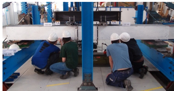
Reinforcement layout and casting of the beams (left) and MSc-students studying the formation of cracks during a full scale experiment (right)
