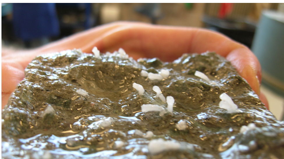
Figure 11: Alkali-silika "worms" swelling out from concrete tested in lab: The chemical reaction releases silika (SiO 2 ) in the aggregates and creates alkali-silika gel. The gel can absorb water and expand, and the concrete may crack.
