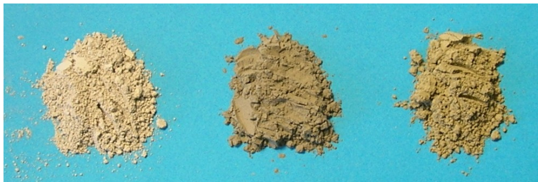
Figure 13: Ground limestone, fly ash and clinker – components in cement
