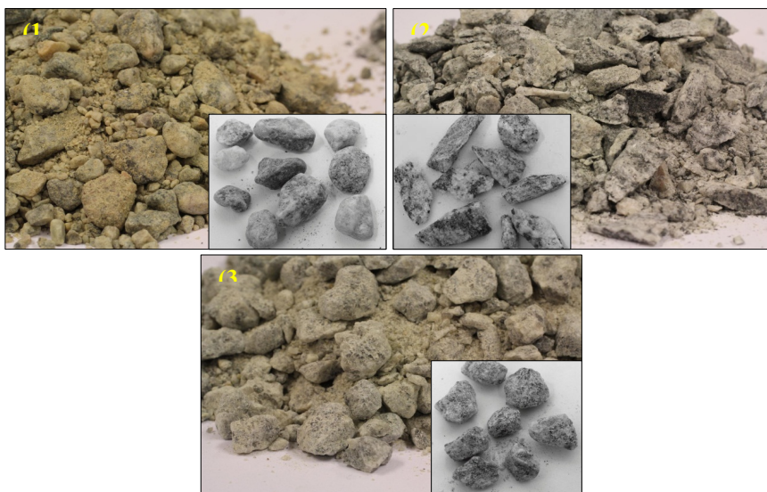
Figure 10: Different sand types: (1) High quality 0/8 mm natural sand from Årdal; (2) Low quality 0/8 mm by-product of coarse crushed aggregate production (should not be called manufactured sand); (3) High quality 0/8 mm manufactured sand.
