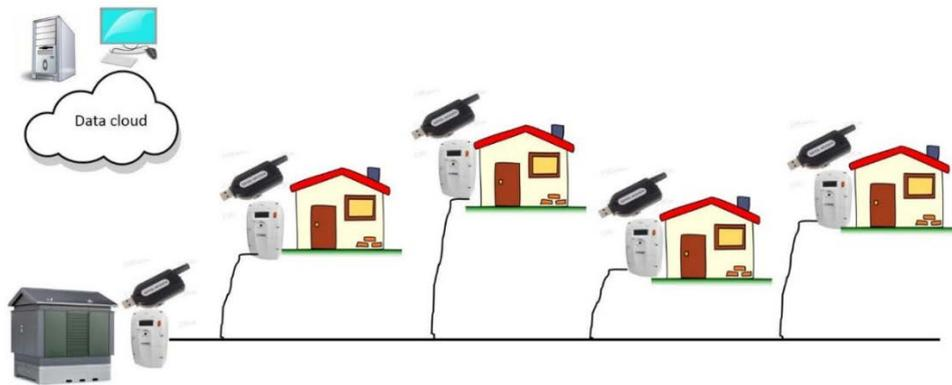
*Transformer station with connected houses, all with smart meters transferring real-time data via modems to a cloud service for analyses.*
