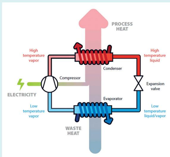
*Simplified illustration of a vapor compression heat pump – Source: de Boer et al., 2020, Strengthening Industrial Heat Pump Innovation – Decarbonizing Industrial Heat (whitepaper).*
