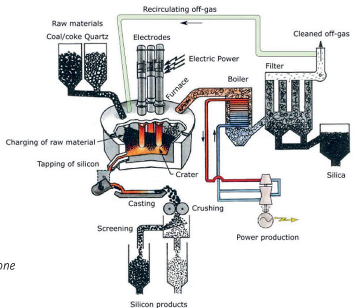
*Illustration that shows how recirculating off-gas can be done in the silicon production process. Illustration modified. Illustration: Halvard Tveit, Elkem (CC BY-SA 4.0).*
