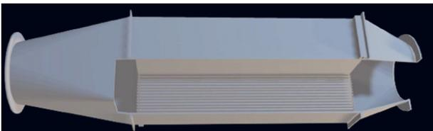
low velocities at the inlet, to avoid particles entering further into the heat exchanger – but for good heat transfer properties, the gas should accelerate once inside.
