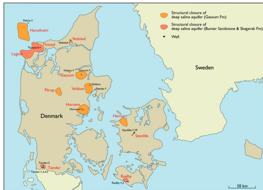
Figure 5-1 Map showing the position and outline of structural closures. Black dots indicate the position of some of the deep exploration wells used in the evaluation of the reservoir formation. For the Hanstholm structure was used 3 additional wells from the offshore area.
