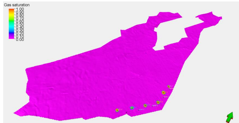
Figure 7-9 CO 2 distribution at top Faludden after 10 years injection showing position of injection and production wells.
