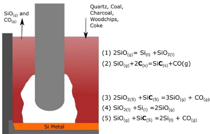
Figure 1- Schematic of industrial Si-furnace and reactions
