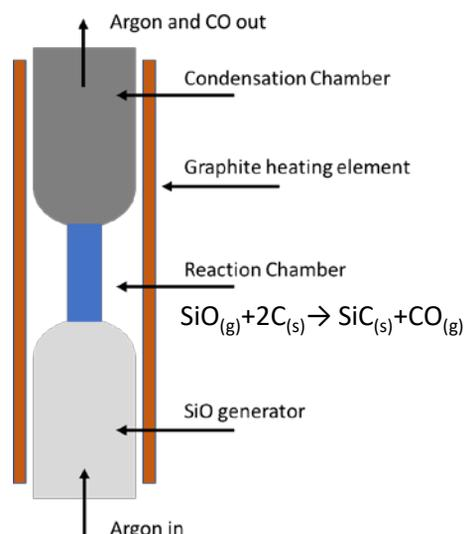
Figure 3- Schematic of the SiO test setup
