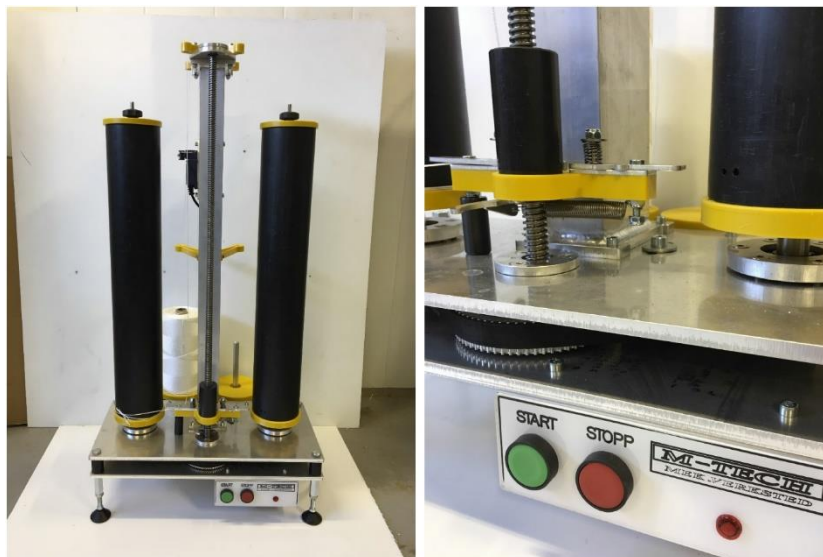
Figure 23. On-spinning prototype of substrate line on plastic cylinders. The cylinders are later placed bioreactors in the lab for the growth-phase
