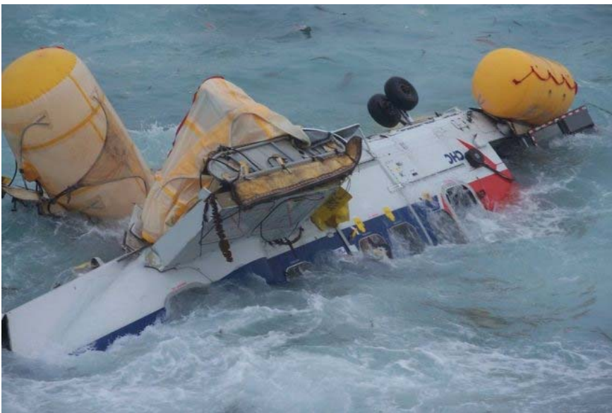
Figure 7.3: Floating devices preventing capsizing will reduce the need for reactive measures (consequence reduction). Picture from the Sumburgh accident in 2013. (Source: The Shetland Times).
