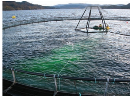
Fig. 4 : Colour dye is distributed in the centre of a commercial cage and dilution measured with time and distance in order to indirectly describe the water flow.
