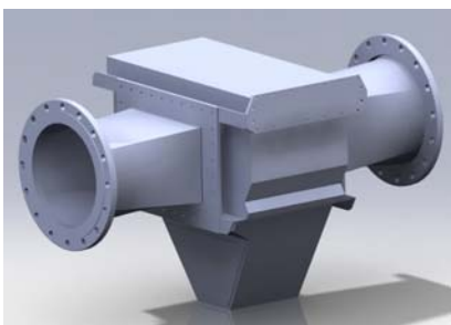
Figure 17. Flatsetsund pipeline counter (Illustration: Flatsetsund).
