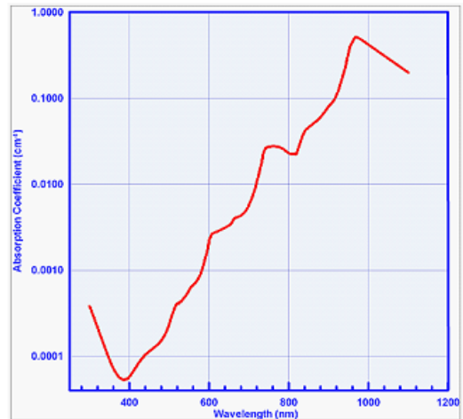
Figure 11. Transmission and absorbance curves for pure water. We should use a wavelength that is invisible for the fishes. But, if also shorter wavelengths than 800 nm is invisible for the fishes we can improve range and image quality by go to shorter wavelengths.
