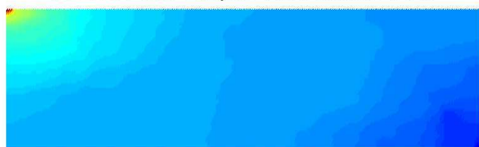
Pressure field computed with mimetic FDM
